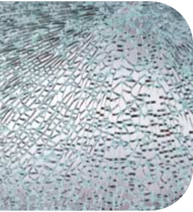
Typical fragmentation pattern of toughened glass
